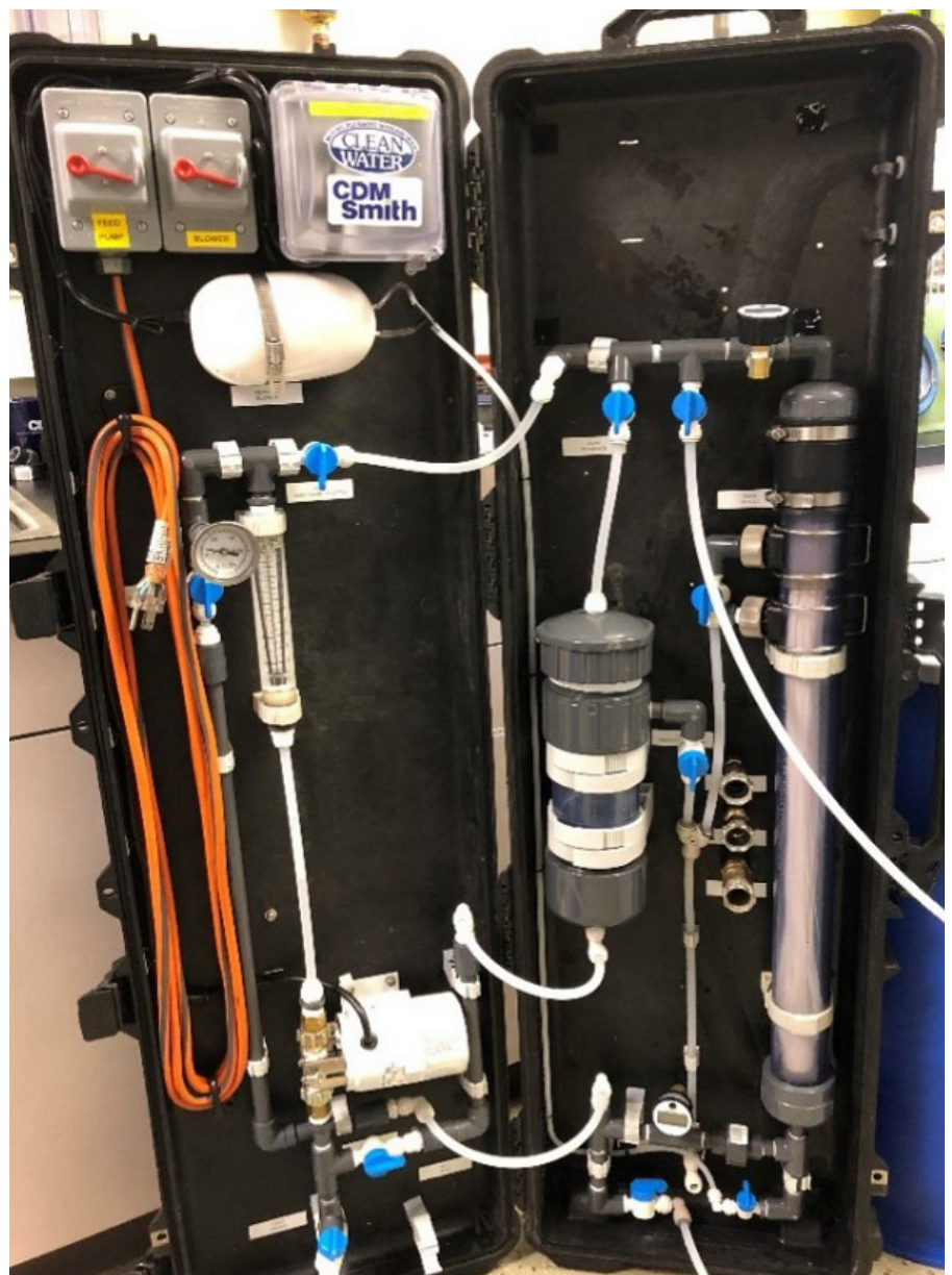
Figure 3. Ultrafiltration Benchtop Unit (Suez ZeeWeed 1500 Jr)
