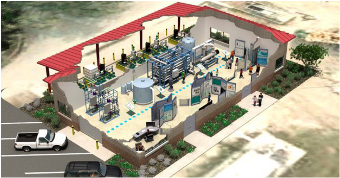
Figure 5. Conceptual Rendering of Mount Pleasant Waterworks' Proposed 30 gpm DPR Demonstration Facility
